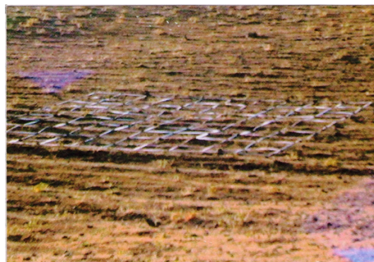
Fig. 3. White fences for measuring degradation of vegetation on slopes.
