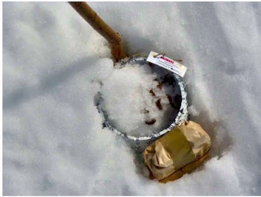
Fig. 3. The collection of fecal pellets from each roost was arranged in a 20 cm long and 15 cm diameter piece of pvc pipe, perforated and painted white to eliminate overheating. A temperature logger, model KTL-108 from Keytag wrapped in beige-colored paper was situated adjacent to the pipe in order to record when the collection of pellets emerged at the snow surface (indicated by alternating day/night temperature) during the spring snow melt.
