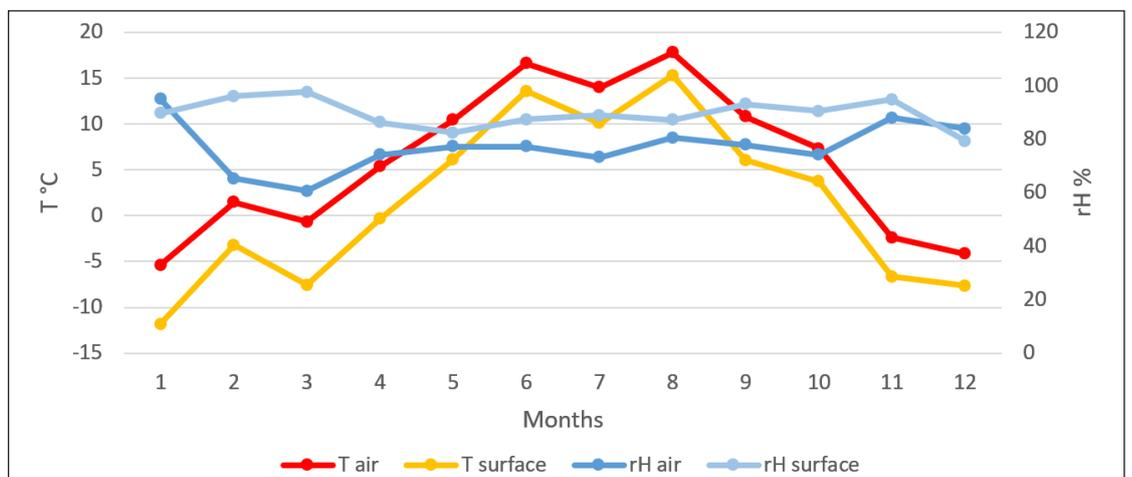
**Fig. 8.** Annual air and surface temperature (T) and humidity (rH) in both study sites (L1 and L2). Average values represent four measurements from individual parts of the day (morning, afternoon, evening and night) during survey (from October 2021 to October 2023).
